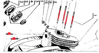
In the motorcycle engine, the stud is screwed into the crankcase components during manufacture and it is seldom necessary to replace it. However, over time the threads can become damaged or the rod bends. Sometimes it helps the dismantling process if one or more studs are removed. Stud removal is an easy process explained below.
