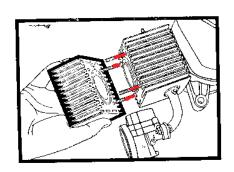
The reason it is necessary to dismantle is to allow you access to fit 2 (two) nuts to the threads on the stud. Sometimes this can be done without dismantling for example with carb studs but on cylinder heads the cooling fins get in the way for the next process. With carb studs they are not usually long enough to allow the fitting of 2 nuts unless you can use thinner nuts. (Thin "Half" nuts are available)
