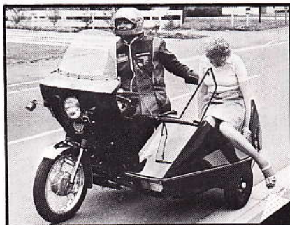
The screen folds forward to make getting in and out easier, but it's still awkward as Liz Kelly discovers.
